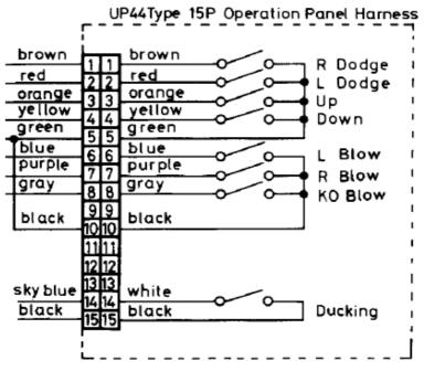
CHPU-41-11 - UP 42 Type Operation Panel Harness (Punch-Out!! and Super Punch-Out!!)
