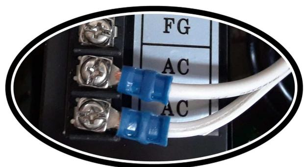
Attach the blue spade connectors to the two A/C lugs of the new switching power supply.
