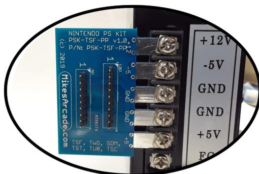
Matching +5, GND, -5 and +12 lugs with the supplied switching power supply.
