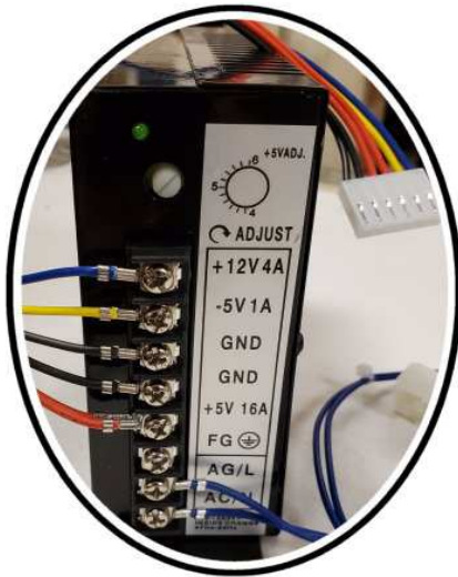
6 PIN DC POWER HARNESS D +5V ( both), BLACK GND, YELLOW -5V, BLUE +12V
