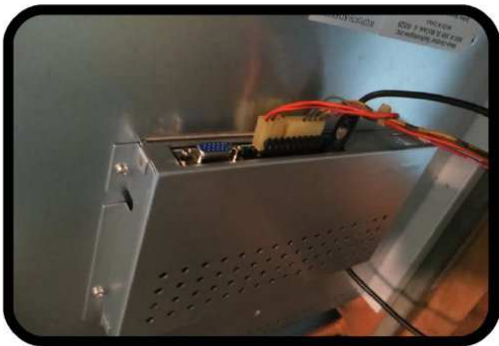
Video signal and Power connections
