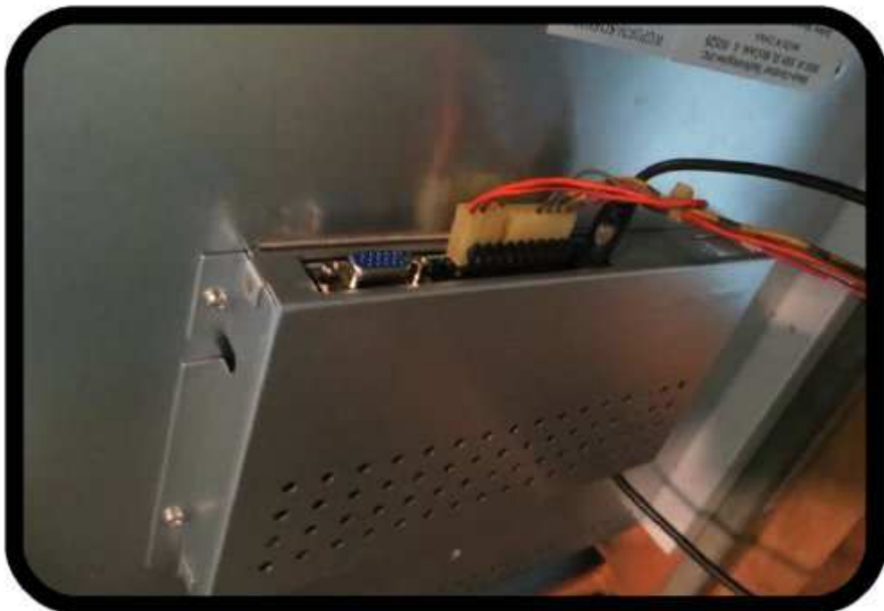
Video signal and Power connections
