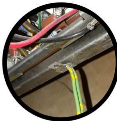
Locate and disconnect the green and yellow wire ground strap (if attached to the monitor frame)
