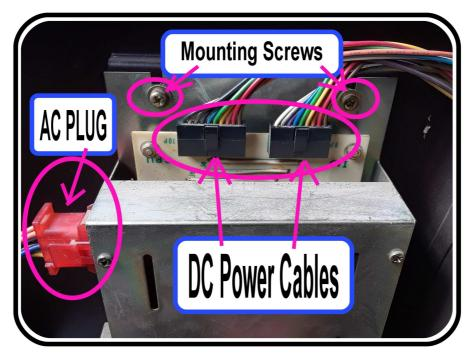
3. Assemble the new power supply and mount it where desired.
