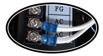
Attach the blue spade connectors to lugs with the supplied switching the two A/C lugs of the new switching power supply.
