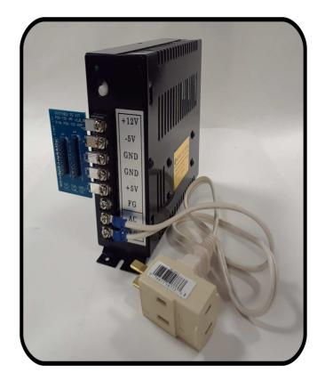
The kit includes a power supply, interface adapter & AC power tap.
