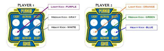
ONCE ALL 6 KICK WIRES ARE CONNECTED TO THE CORRECT BUTTONS, YOU MUST NOW INSTALL THE BLACK GROUNDING WIRES FOR EACH BUTTON.
